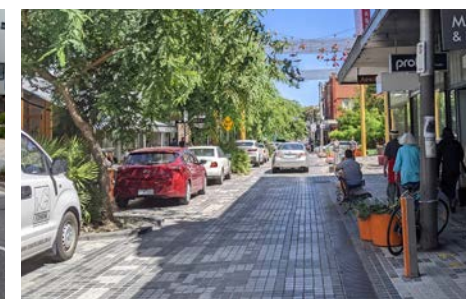
Image 12. Slow speed surface treatment and canopy trees in curb outstand.
